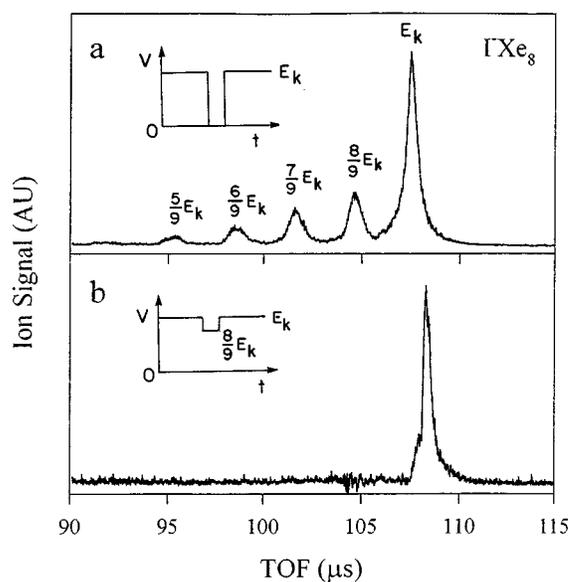
FIG. 1. A reflectron MS spectrum of the  $\Gamma^-Xe_8$  (a) together with its daughters, after being selected by a conventional stopping MG, and (b) with no daughter peaks, after being selected by the MG-energy discriminator.
